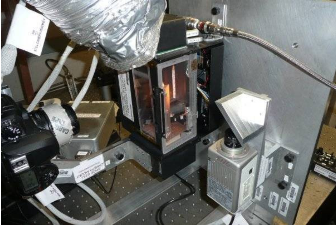
Figure 3.7. SPICE prototype module operating at the University of Maryland FETS Lab. Exhaust and camera systems are visible.
