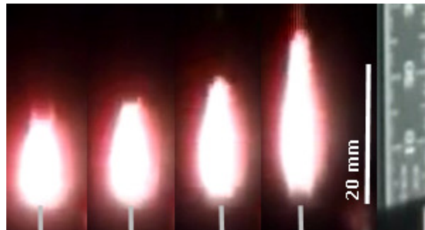
Figure 6.8. Stills of smoke points and measurements for 75% propylene, 0.762 mm burner. Rule image taken for reference is also shown.
